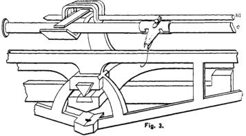
the movement, the rider is left hanging free upon the beam. Upon releasing the rod, c, the tension of the spring should be sufficient to close the forceps. When, however, it is often desirable to leave the rider upon the beam, by bending its loop, as shown in the side sketch, Fig. 2, this is easily effected.
